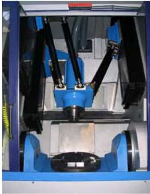
Figure 1.8- Machine-outil Verne de Fatronik.
